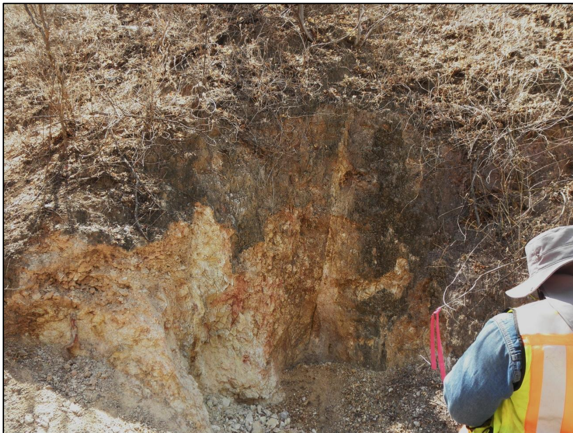
Figure 3. Outcrop sampling north of exposed ridge with high grade Au 9.56 g/t and Ag 515 g/t – sample 221009 showing intense zeolite, clay and jarosite alteration of andesite
