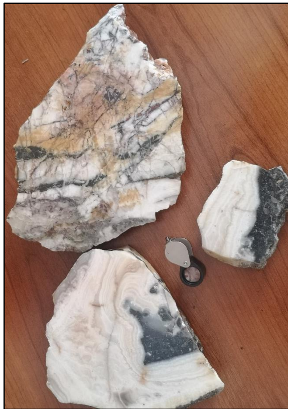
Figure 5. Polished samples showing epithermal chalcidonic silica veining with complex depositional and compositional banding, open space filling and multi-stage brecciation from Mystery property.
