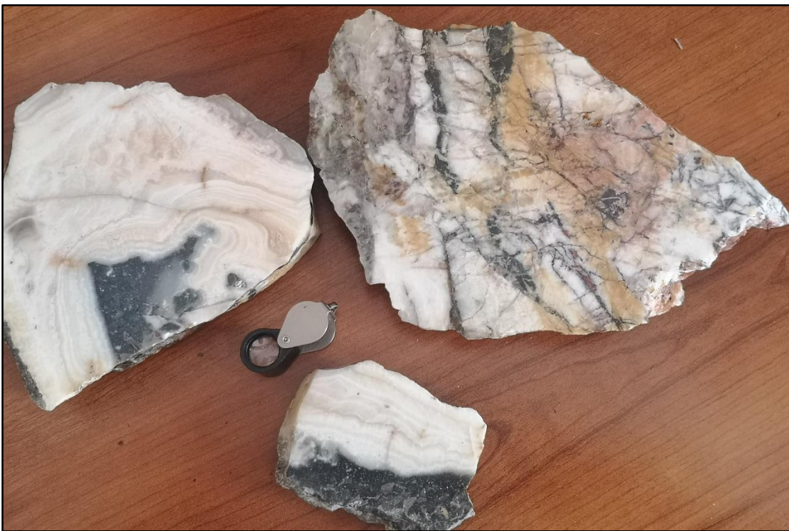
Figure 3. Silica veining with complex deposition as fine laminations to coarse crustiform textures, compositional and textural banding, and multi-stage or episodic brecciation and infilling from Marilyn property.
