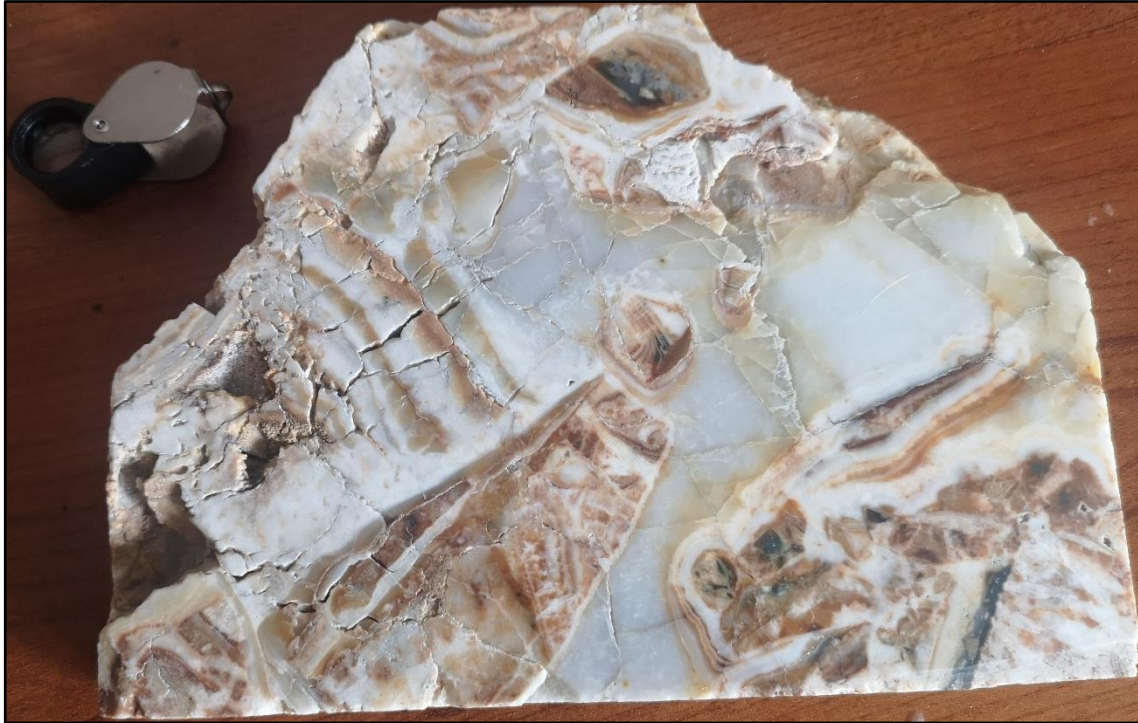
Figure 2. Epithermal chalcedonic silica veining with complex depositional and compositional banding, open space filling and multi-stage brecciation from Mystery property.
