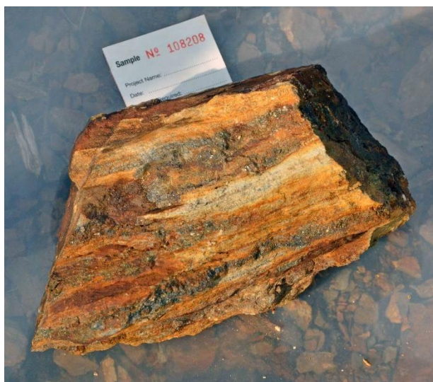
Photo 21. Sample of intensely altered, ferroan sphalerite-rich sericite schist at Relf Zone
