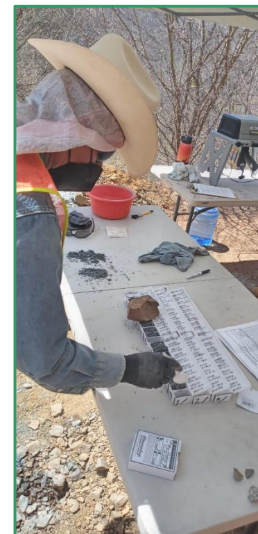
Chip logging with portable XRF in background
