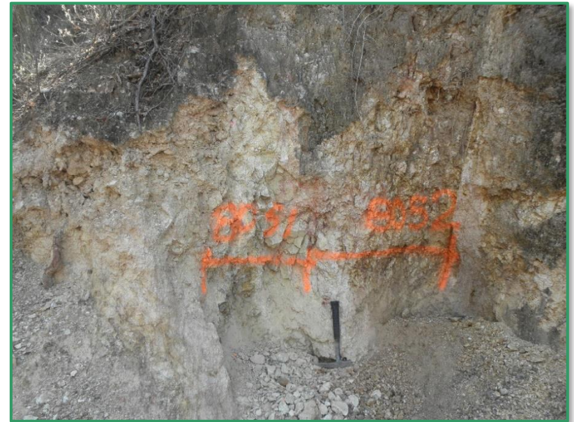
Phase 1 sample pit 9.56 g/t Au, 515 g/t Ag Intense zeolite, clay, jarosite 'argillic' alteration
