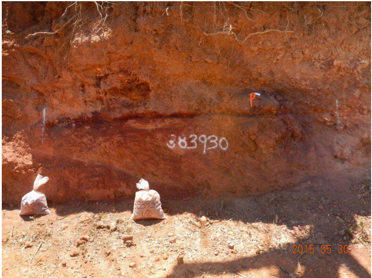
Figure 18. Sample 383930 from new road cut in gossan area; 3.3 m @ 0.054 g/t Au, 20 g/t Ag.
