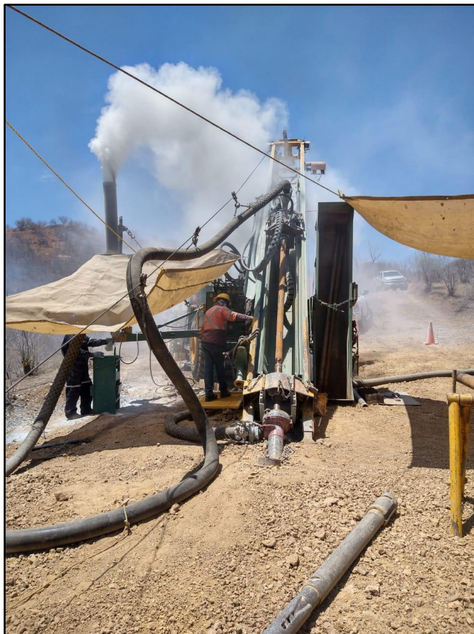
Figure 1. Looking north across Pad M1 (MEZ001, MEZ-002, MEZ-003) at El Mezquite showing RC rig from Layne de Mexico drilling on a southerly azimuth at -45° dip angle
