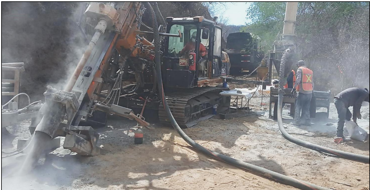
Figure 1. Reverse circulation drill rig collared on pad #40 north of artisanal underground workings at the Pillado drill target, first DDH on the Diamante 1 concession.
