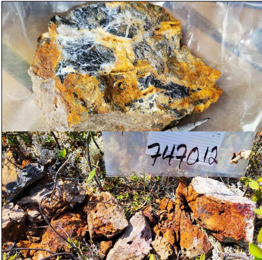
Figure 4. Marilyn sampling from southern cluster (747011 - top, 747012 - bottom) showing brecciation, episodic massive to vuggy silica veining and surface oxidation of sulphides including arsenopyrite.
