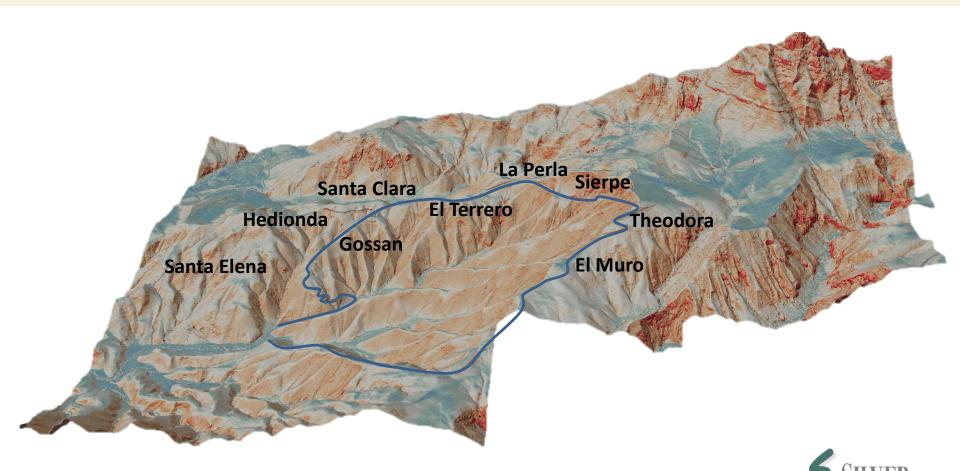
LiDAR enhanced digital elevation map with drill targets looking south across Pino de Plata property
