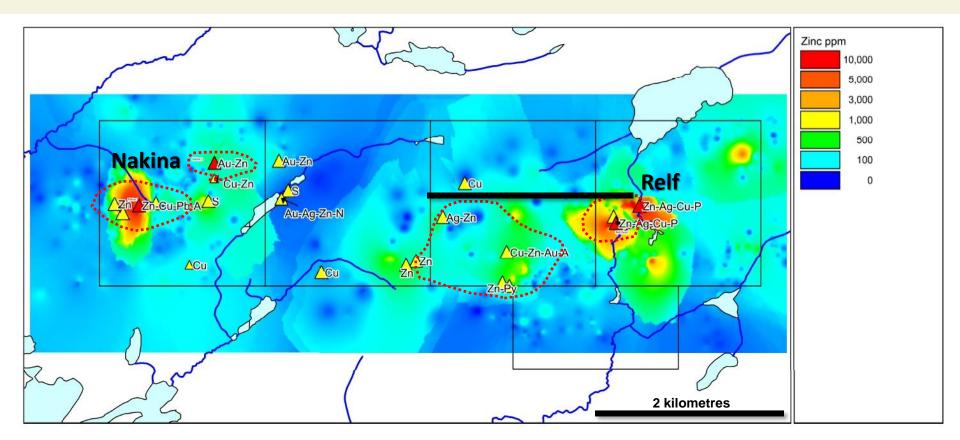
Contoured zinc analyses from grab rock samples from principal targets. Shallow drilling in western Nakina target. Mainly shallow with two deeper holes at eastern Relf Lake target. Note 10,000 ppm Zn = 1% Zn.
