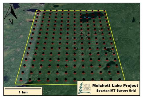
SPARTAN MT is a robust full-tensor audio-magnetotelluric technology that acquires high quality data in the 10 kHz to 0.001 Hz frequency band. MT is a passive electromagnetic geophysical technique that uses natural electric fields from lightning sources, solar flares and ionospheric resonances that induce current flow in the ground which may be used to image the earth's electrical resistivity structure from surface to great depths.
