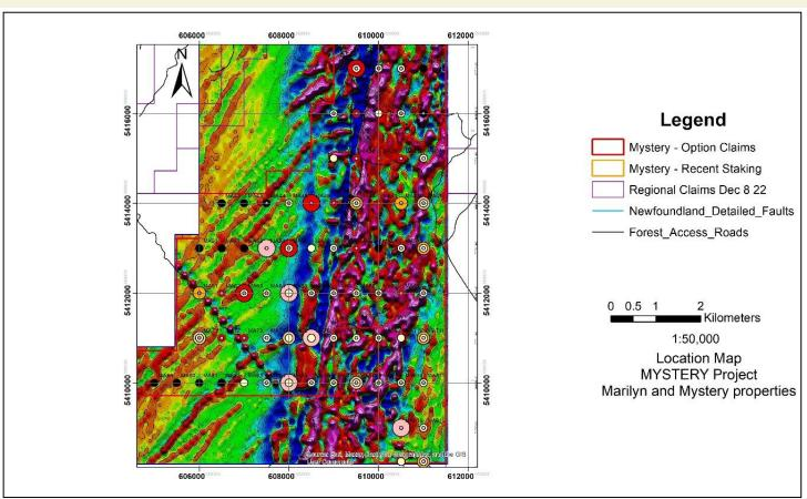
Map of the Marilyn claims showing combined gold grain frequency and heavy metal geochemical signature anomalies upon airborne geophysical map – first vertical derivative. Botwood Group metasediments on west with northeast fabric in contact with north-south Mount Peyton multi-phase intrusion to the east. Black dots denote unsampled sites. Powerline crosses to SE.
