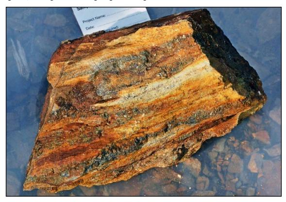
Figure 3. Zinc (Fe-sphalerite) mineralization in quartz-sericite-pyrite schist collected by Project QP from the main trench in the Relf Lake Zone.
